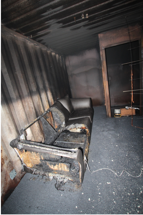
Figure 5.27: Photographs of the fire damage to the sofa from Experiment 1.
