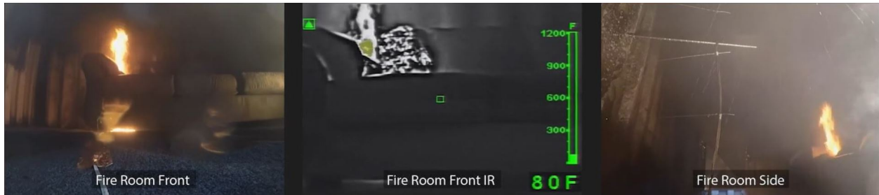
Figure 5.14: Experiment 3 - Conditions in the fire room at 205 s, 30 s after nozzle activation.
