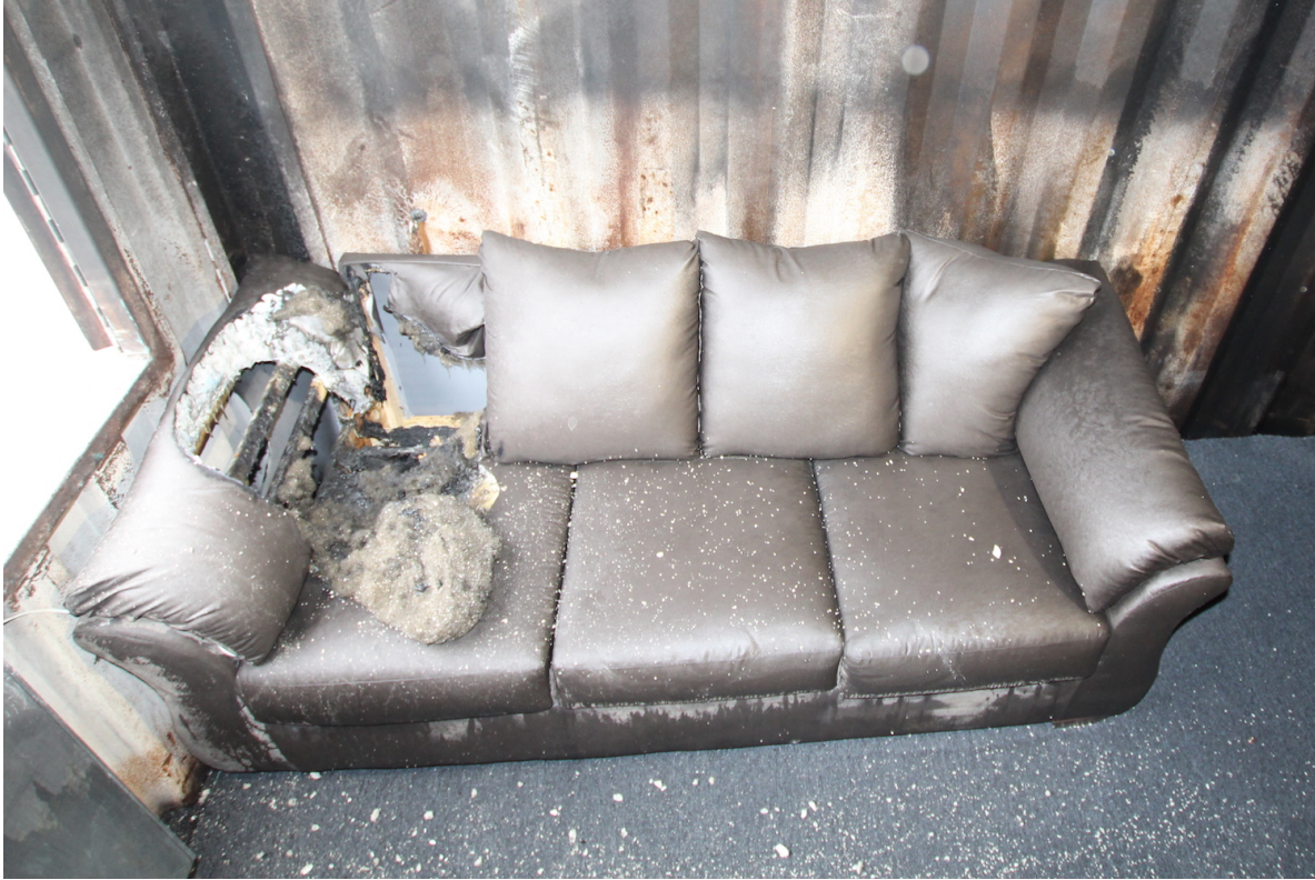
Figure 5.30: Photograph of the fire damage to the sofa from Experiment 4.
