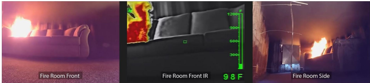
Figure 5.18: Experiment 4 - Conditions in the fire room at 135 s, just prior to nozzle activation.
