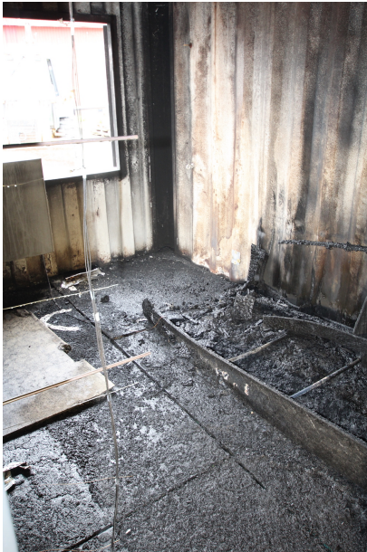
Figure 5.31: Photographs of the fire damage to the sofa from Experiment 6.
