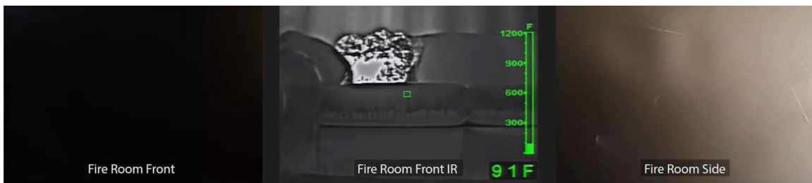
Figure 5.10: Experiment 5 - Conditions in the fire room at 165 s, 30 s after nozzle activation.
