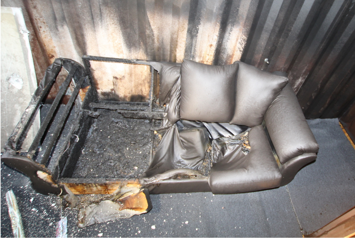
Figure 5.29: Photograph of the fire damage to the sofa from Experiment 3.
