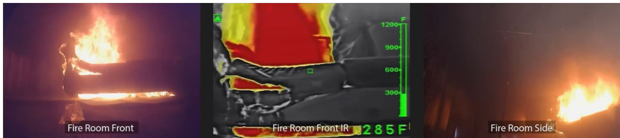
Figure 5.15: Experiment 3 - Conditions in the fire room at 420 s, 30 s before the nozzle water flow was increased.
