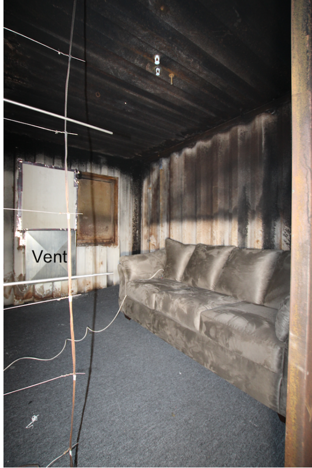
Figure 3.5: Photograph of fire room with furnishings installed.
