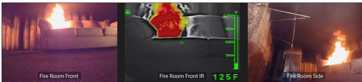
Figure 5.9: Experiment 5 - Conditions in the fire room at 135 s, just prior to nozzle activation.
