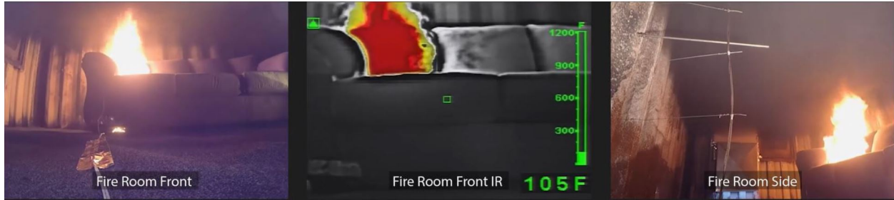
Figure 5.13: Experiment 3 - Conditions in the fire room at 175 s, just prior to nozzle activation.
