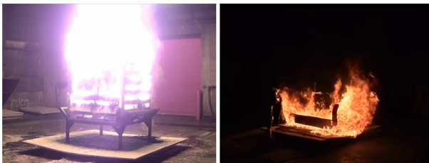
Figure 8. Visual comparison of six pallet boxed-in triangle (6P1S-BT) and upholstered sofa (SCI) fuel package experiments at time of peak HRR (3.6 MW and 3.7 MW, respectively).
