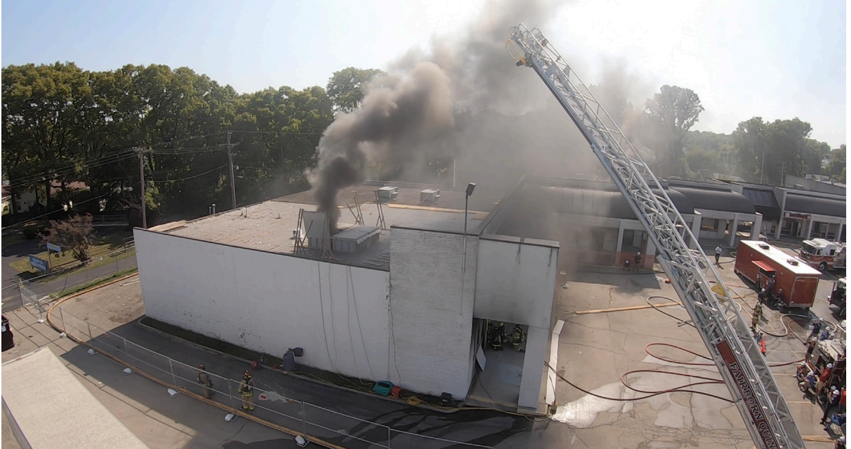
Figure 12: Exterior conditions through the open vertical vent and at the front door following initial suppression.
