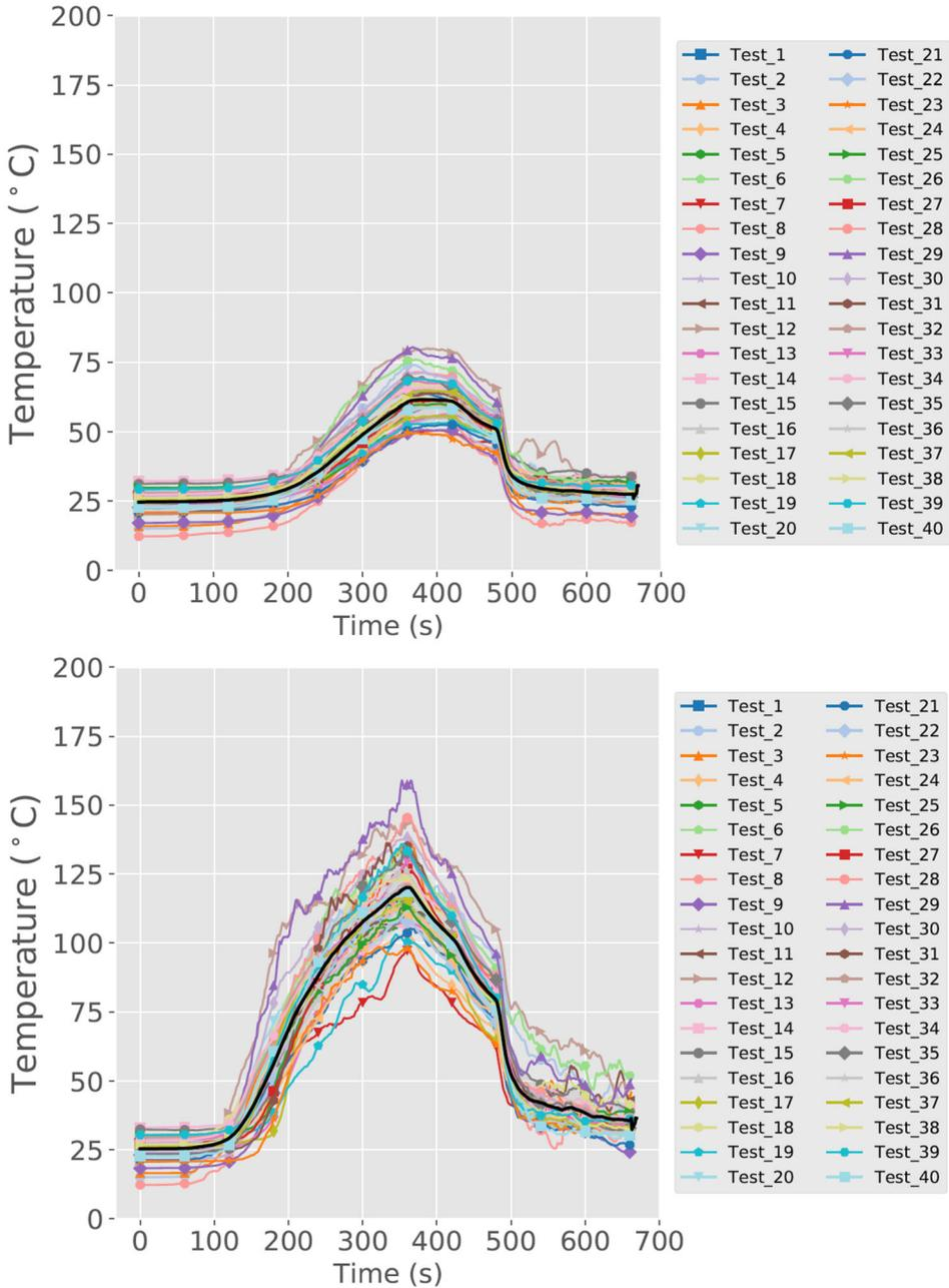
**Figure 2. Temperature profiles from 40 separate burn trials at (top) 0.9 m from the floor and (bottom) 1.5 m from the floor. Data collection begins upon ignition and the fire grows until suppression at 360 s followed by opening the exposure chamber doors at 480 s. The black line without markers represents the average of all 40 trials.**
