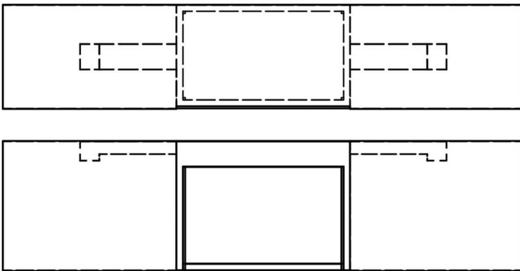
**Figure 1. Fireground Exposure Simulator (FES) prop. (top) Photo of prop being prepared for a mannequin exposure trial, (middle) overhead and (bottom) side perspectives of FES prop showing the combustion chamber in the middle and exposure chambers on each end.**
