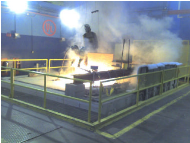
Figure 39 – Picture of one instance where flaming through the floor is visible
