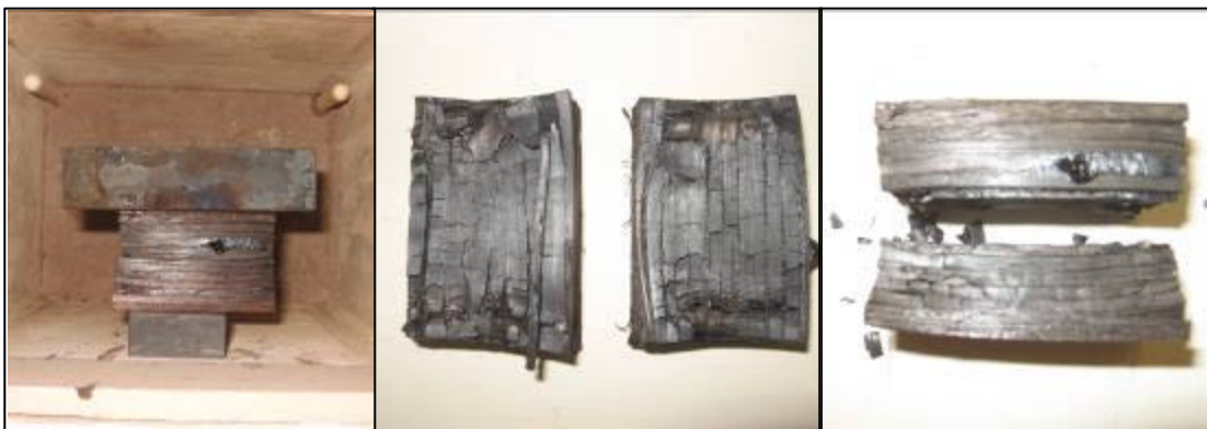
Figure D5 - Charred wood from engineered lumber (Type B) after completion of thermal properties experiment
