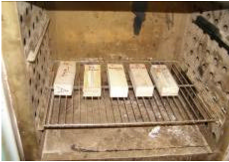
Figure D 13 - Heating the specimen in oven
