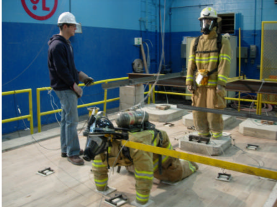
Figure 35 - Picture from test showing floor loads
