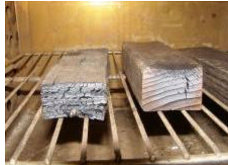
Figure D 14 - Wood charring at 250°C
