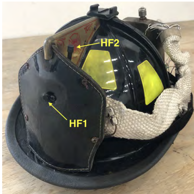
Figure 3.15: Image of the helmet worn by the firefighter at the nozzle during experiments involving interior suppression. Two heat flux gauges mounted on the helmet, labeled “HF1” and “HF2” measured the incident heat flux exposure to the firefighter in the horizontal and vertical directions, respectively.
