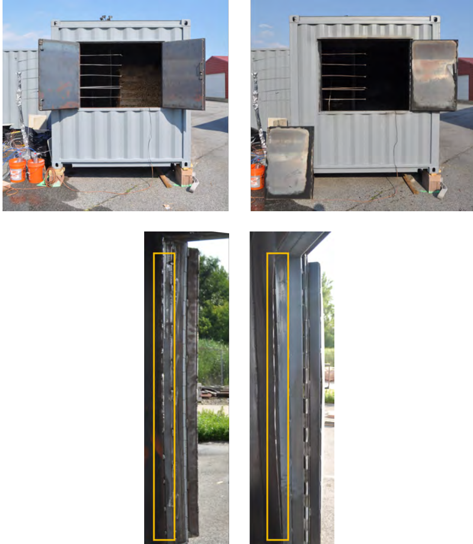
Figure 5.10: Images of the Insulated Metal Prop before (left side) and after (right side) the Burn In experiment. The top images are of the exterior side of the fire room window, and the bottom images are looking at welds along the edge of a steel sheet on the interior side near the window. The left window shutter became detached from the prop, and multiple interior welds were broken as a result of the Burn In experiment.
