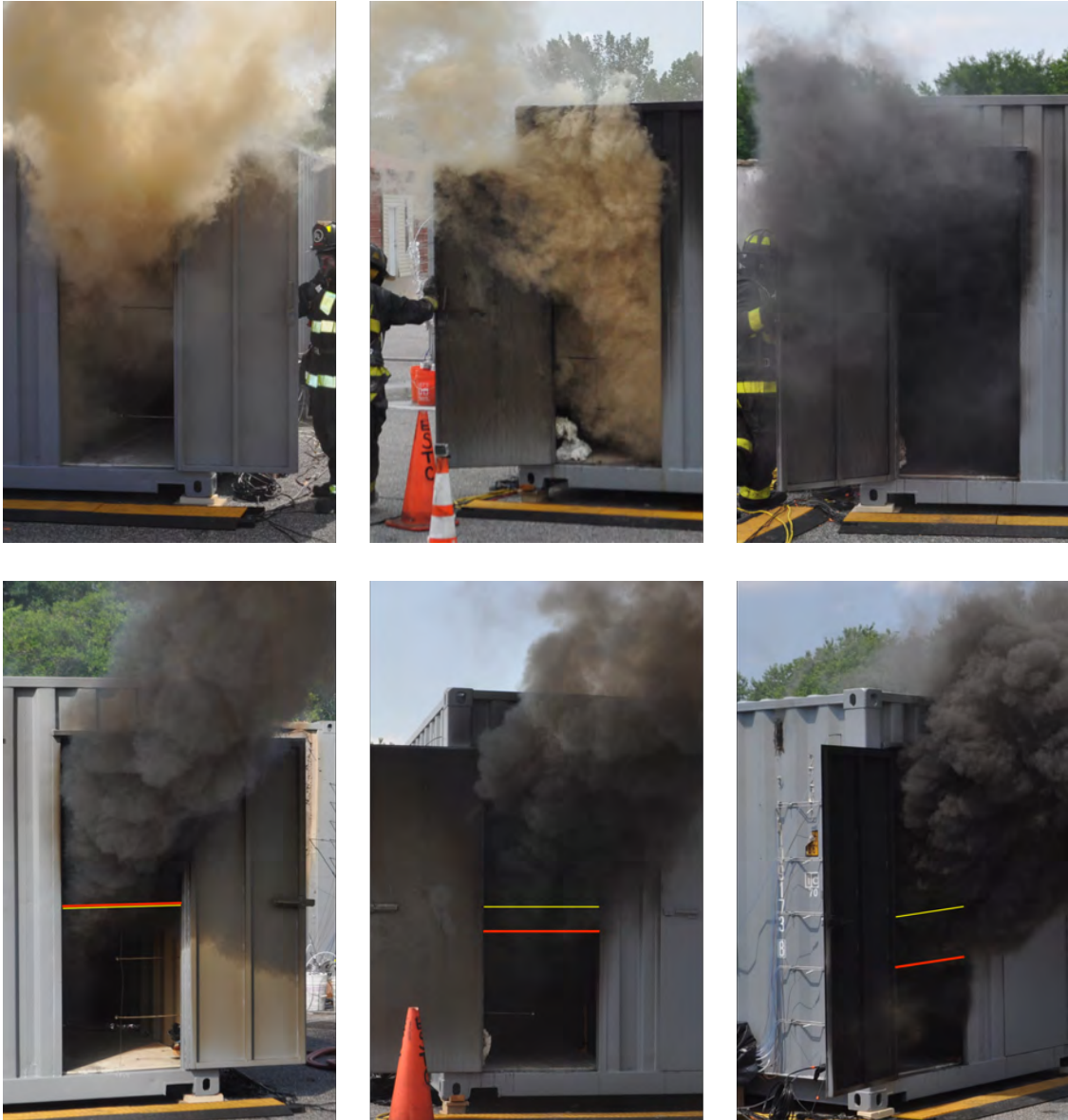
Figure 6.6: Images of the smoke conditions immediately after the hall door was opened (top row) and after the neutral plane developed at the doorway (bottom row) during tests with the pallets (left side); pallets and OSB (middle); and furniture (right side) fuel packages. A red line marks the approximate height of the neutral plane and a yellow line marks the height of the door handle to provide a similar reference point in the photos along the bottom row.
