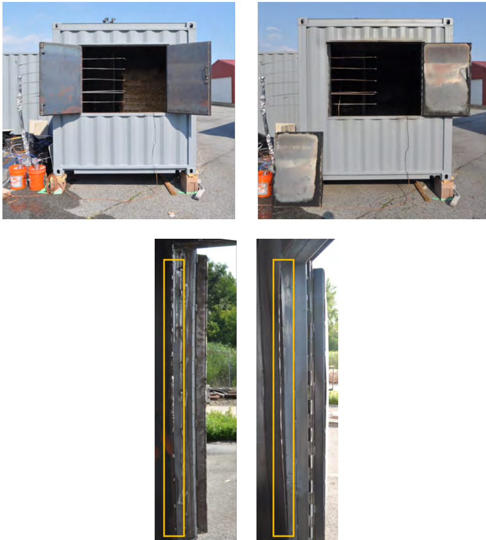
Figure 6.15: Images of the Insulated Metal Prop before (left side) and after (right side) the Burn In test. The top images are of the exterior side of the fire room window, and the bottom images are looking at welds along the edge of a steel sheet on the interior side near the window. The left window shutter became detached from the prop and multiple interior welds were broken as a result of the Burn In experiment.
