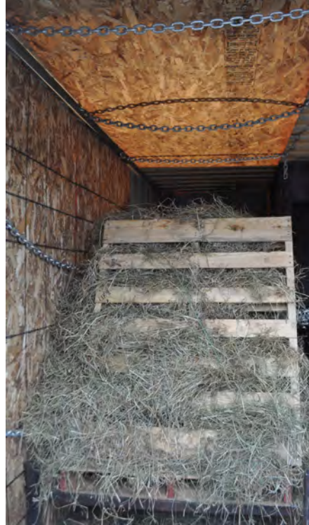
Figure 3.11: Image of the pallets & OSB fuel load.
