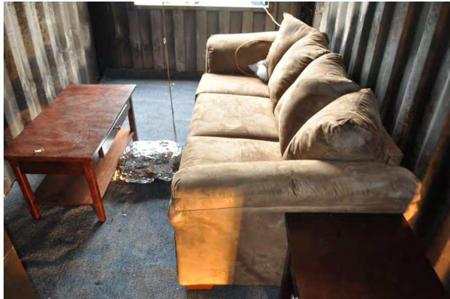
Figure 3.12: Furniture fuel load consisting of a couch, coffee table, end table, and carpet on top of padding and OSB.
