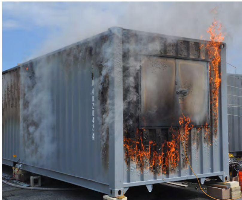
Figure 4.1: Example of fire spread to the exterior surface of the Metal Prop during the initial experiment. This phenomenon was caused by the exterior paint reaching its autoignition temperature and igniting.
