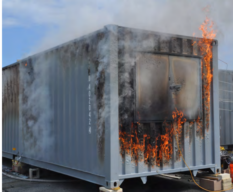
Figure 6.13: Image of fire spread along the exterior surface of the Metal Prop during the Burn In experiment.
