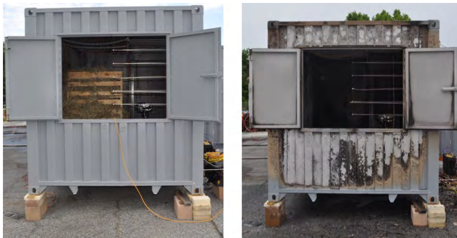
Figure 5.9: Exterior photos of the Metal Prop before (left) and after (right) the Burn In experiment.
