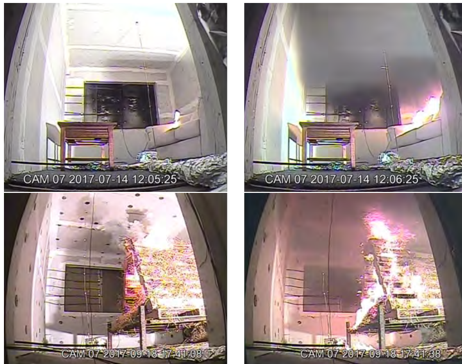
Figure 5.7: Still images obtained from recorded video of fire growth after ignition of the furniture fuel load (top images) and pallets fuel load (bottom images) in the Gypsum Prop. The images on the left side are of times shortly after visible flames were seen in the video, and the images on the right are from 30 seconds later for the pallets and one minute later for the furniture.
