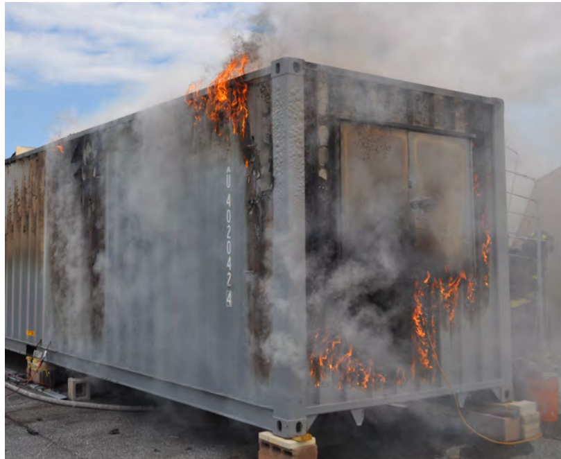
Figure 5.8: Photo of the paint burning on the exterior side of the Metal Prop during the Burn In experiment.
