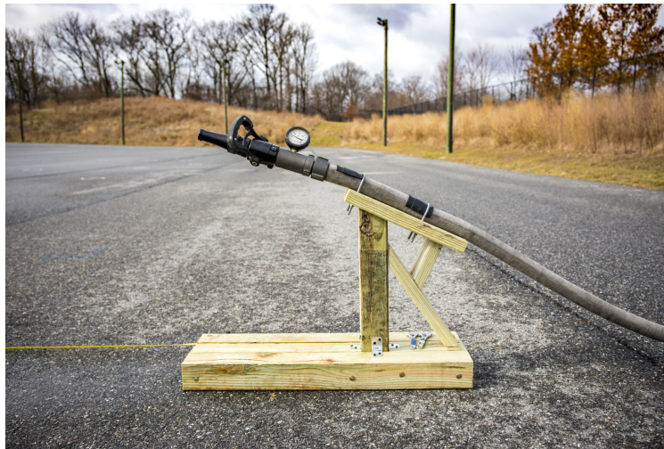
Figure 3.5: Nozzle prop in use for a fixed pattern flow.
