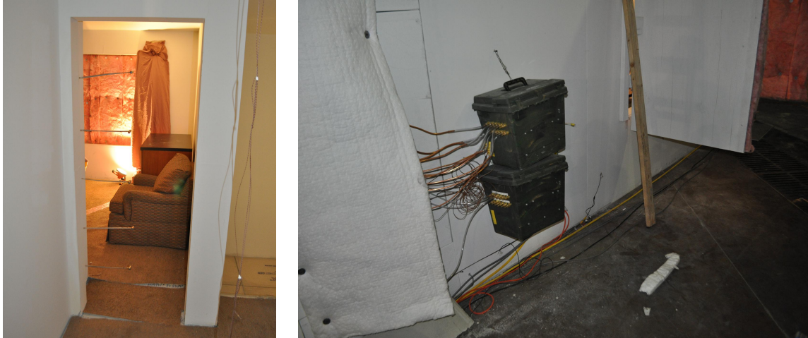
Figure 4.17: Bi-Directional Probe Array. Example of probes in a doorway (left), pressure transducer box (right).
