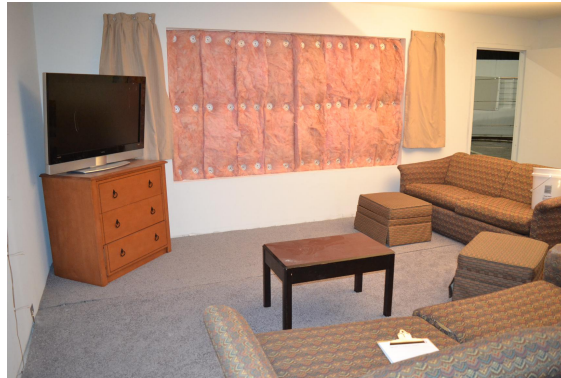
Figure 4.10: Living Room Fuel Configuration
