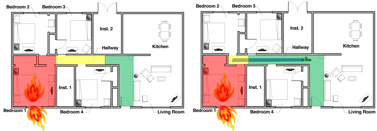
Figure 7.8: Thermal conditions before (left) and after (right) water application down the hallway during an interior suppression tactic. Color conditions represent operating zones per Utech [31] where green is routine, yellow is ordinary, and red is emergency. (Experiment 7)
