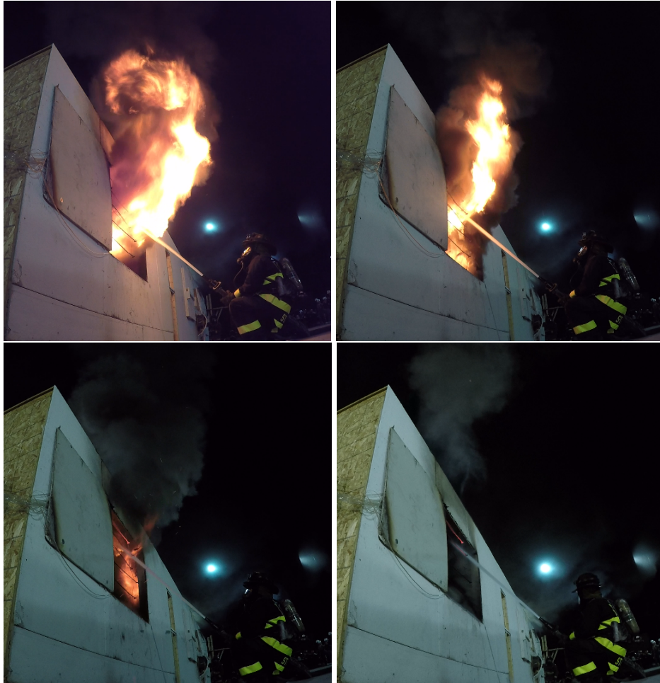
Figure 7.3: Example of the improved conditions from the initial water application during a transition attack using a smooth bore nozzle at a steep angle directed off the ceiling (Experiment 18). Sequence of images is the first three seconds after initial water application. The moment suppression starts (top left), 1 second after suppression starts (top right), 2 seconds after suppression starts (bottom left), and 3 seconds after suppression starts (bottom right).
