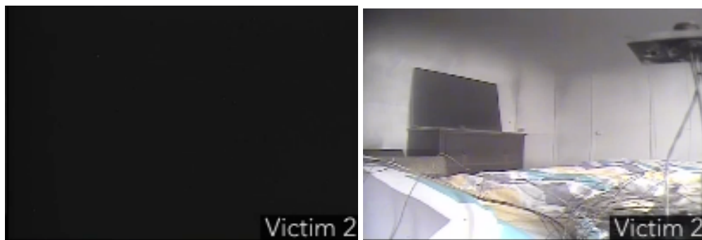
Figure 7.11: Visibility at Victim 2 at 6 min for open door (left) and closed door (right). (Experiment 1 & 2)
