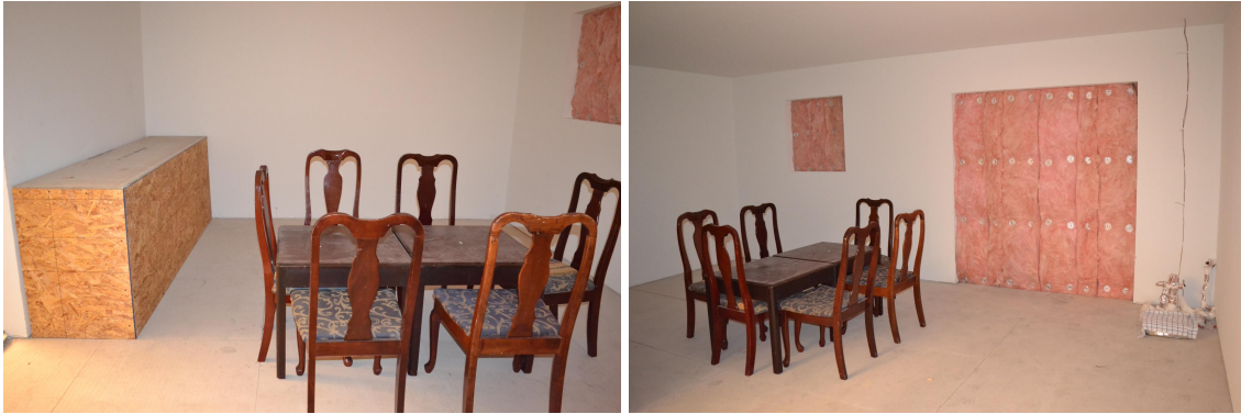
Figure 4.9: Kitchen Fuel Configuration
