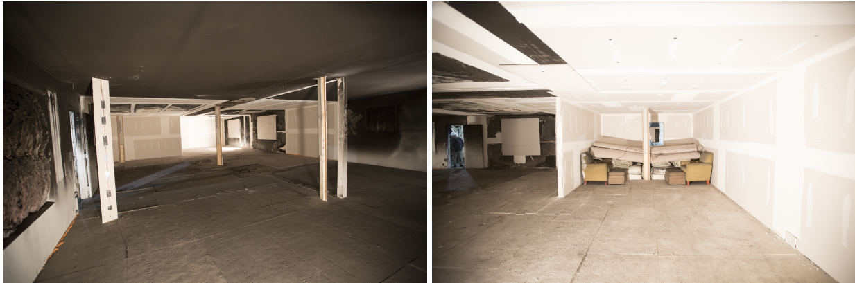
Figure 5.9: Images of the structure configuration, open space (left) and fire room (right)
