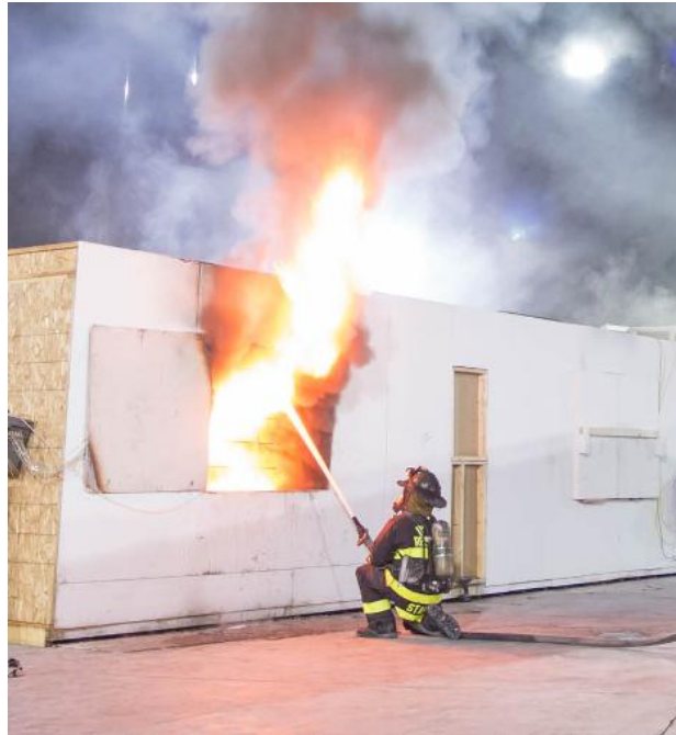
Figure 7.13: Exterior water application using a steep angle off the ceiling.
