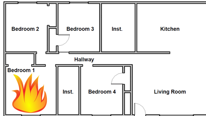
Figure 6.6: Ventilation Configuration - No Ventilation (Experiments 1-6)
