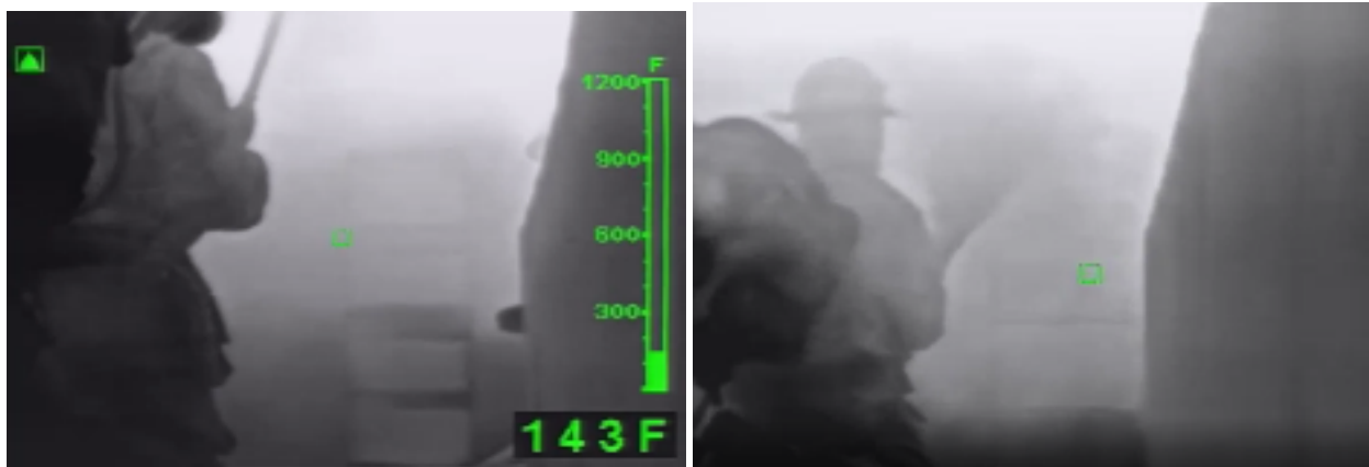
Figure 7.30: Thermal imager views of the two patterns utilized during burst suppression smooth bore (left) and narrow fog (right).
