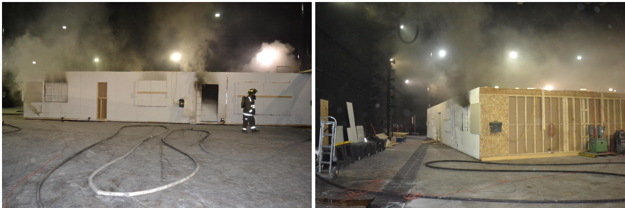
Figure 7.1: Example of no fire showing with no open vents on a residential structure. Side A (left) has a front door and A/B corner window with smoke showing. Side C (right) shows darker smoke showing from the B/C corner. The fire is located in Bedroom 1 in the A/B corner of the structure.
