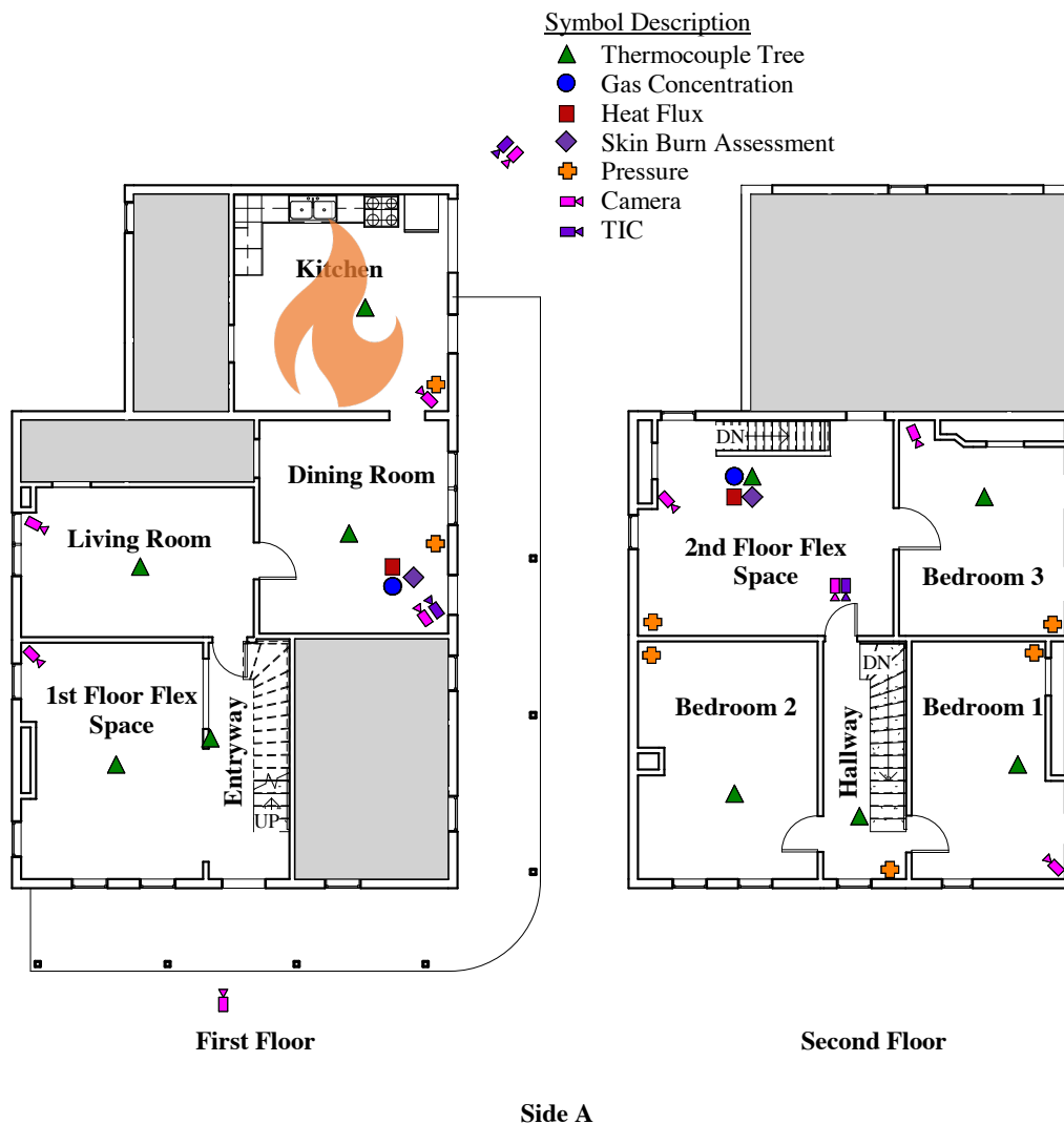
Figure 3.217: Instrumentation and floor plan for Experiment 18. The gray areas were isolated from the remainder of the structure and utilized as space for instrumentation.
