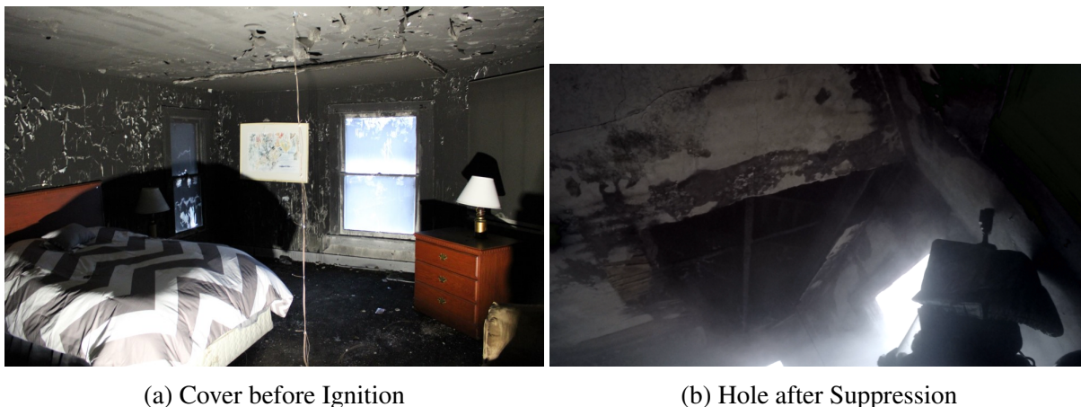
Figure 3.152: Interior photographs of the failed ceiling prior to ignition (see Figure 3.152a) and after suppression (see Figure 3.152b) for Experiment 13.
