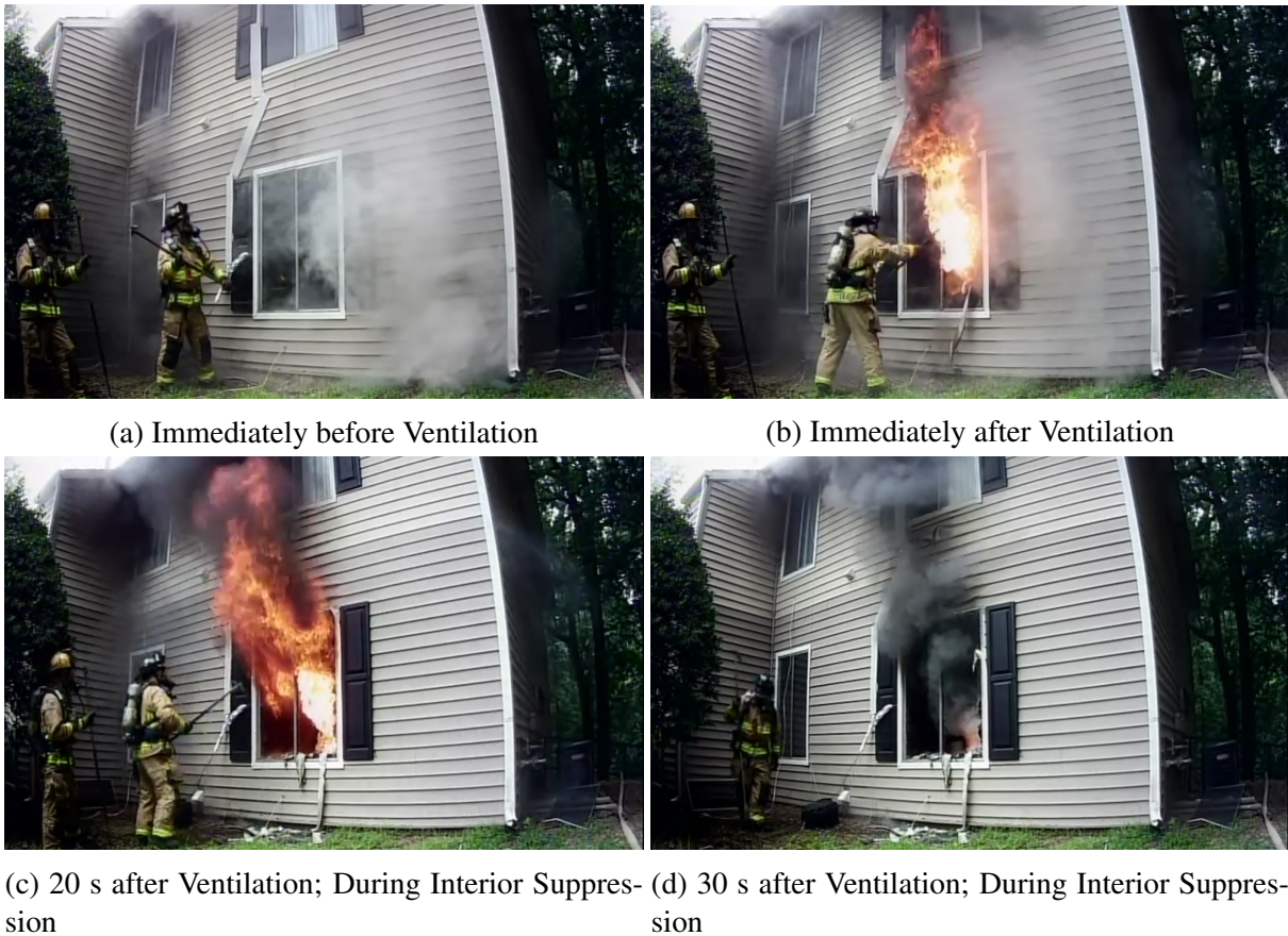
Figure 3.38: Images of the fire room (bedroom) window in Experiment 1D being broken to provide horizontal ventilation in coordination with interior suppression.
