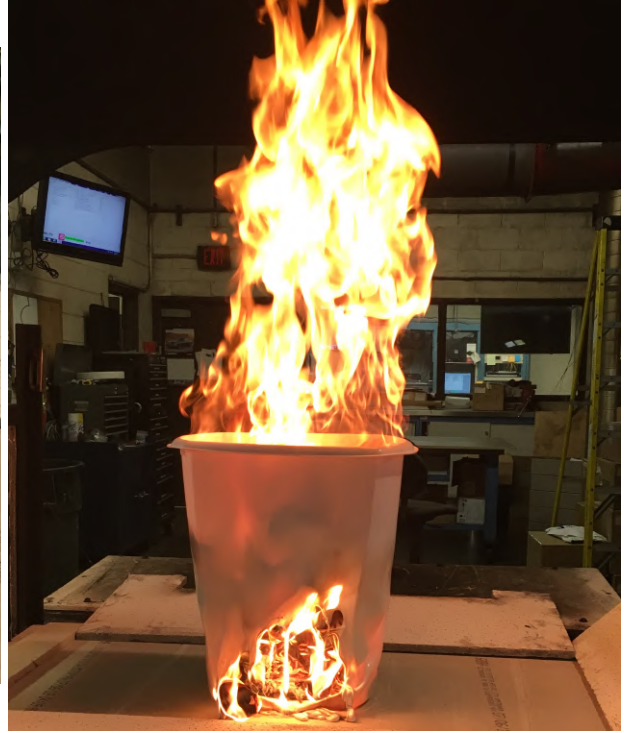
(b) HRR Testing of Waste Container
