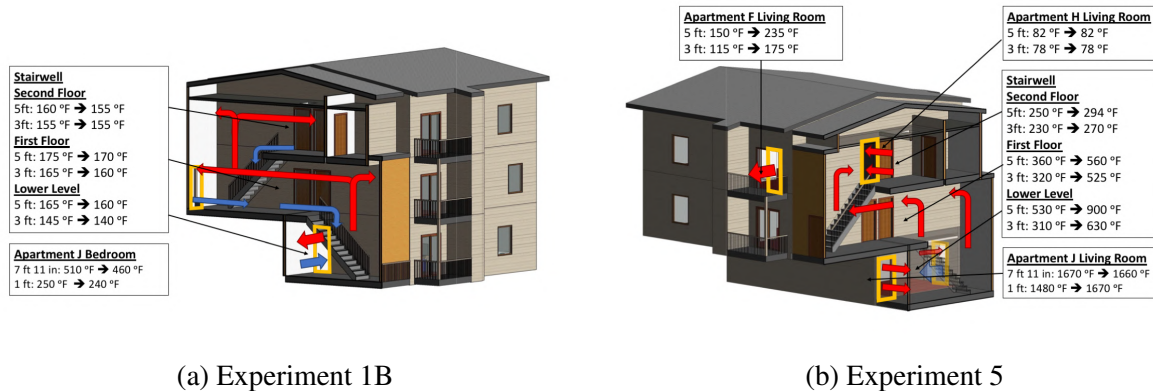
Figure 4.22: Fire apartment and stairwell temperatures for Experiments 1B and 5. Experiment 5 includes target apartment (F and H) living room temperatures. Data are presented from 600 s–630 s post-ignition for Experiment 1B following the stairwell door being opened and from 417 s–447 s post-ignition for Experiment 5, which was after the Apartment F sliding glass door was opened. Red arrows indicate the flow of combustion products, blue arrows indicate the flow of fresh air, and the size of the arrows indicate the relative magnitude of the flow. Yellow boxes indicate ventilation openings.
