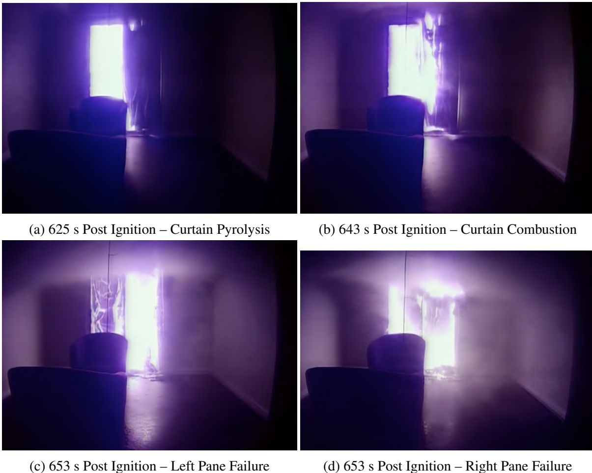
Figure 4.28: Ignition of the curtains in Apartment C prior to the sliding glass door breaking, and an interior view of the living room sliding glass door failing.
